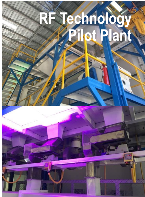
A pilot plant for radio-frequency insect and egg extermination technology. @NSP (Chiang Mai)
